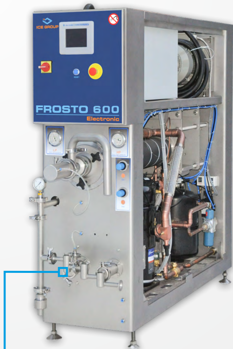
FROSTO 600 version with hermetic compressor
