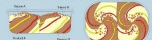
Filling based on 2x STAR 3000 dozers with rotation - 2 ice-creams with radial partitioning and rotation + 2 sauces
