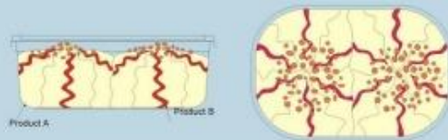
Filling based on 2x STAR 3000 dozers without rotation 2 ice-creams and 2 sauces
