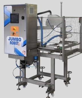
Jumbo Robot – ice cream tubs dosed by means of a robot
