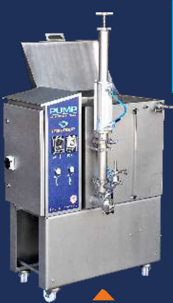
Injection, time operated, pump with heated hopper
