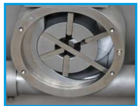
Paddle-type mixing pump, easy to disassemble and servicing
