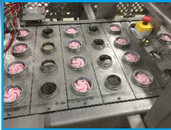
▲ 4-wide in-line machine for Ø75mm and Ø95mm cups
