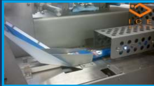
▲ wrapping foil forming on folding box
