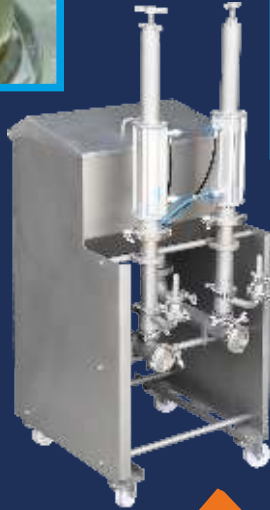
Two injection pumps with divided hopper for two syrup colours
