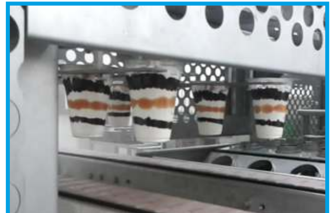
▲ Transfer robot to outfeed conveyor
