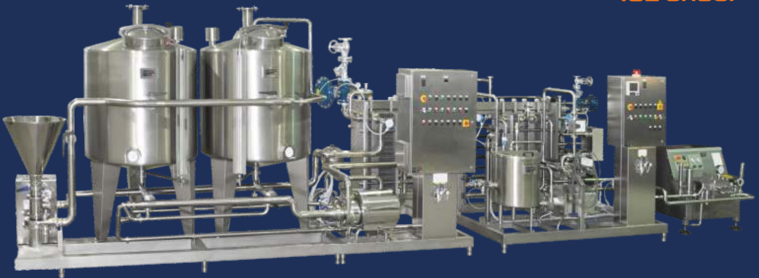
▲ Complete HTST pasteurisation plant with triblender, dissolving unit and homogenizer
