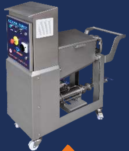
Worm pump (screw type) for continuous feeding of syrup, also with fruit pieces
