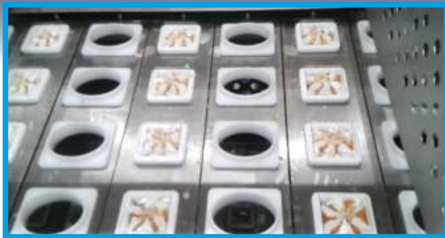
4-wide in-line machine for oval and cubic cups
