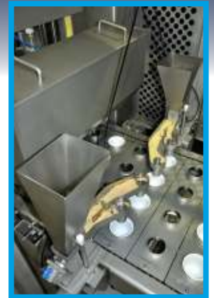
▲ Vibration unit for dry ingredients
