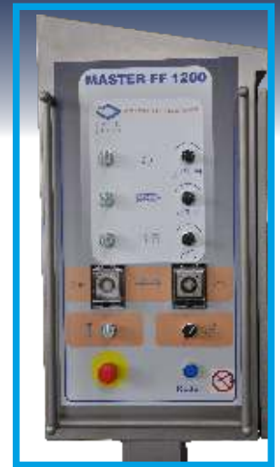
Basic version electric panel with potentiometers (instead of PLC) for controlling 3 motors
