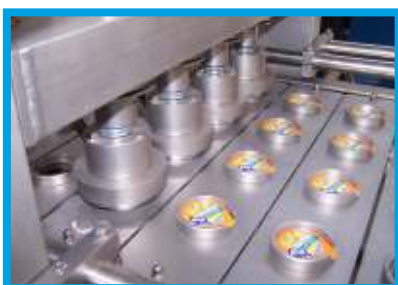
Expert LVF 4 for squeeze-ups with sealing station
