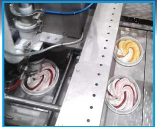
3-axis servo-driven dosing unit
