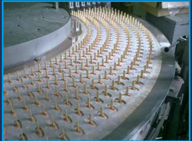
▲ Mold strips and segments for every linear and rotary stick novelty system
