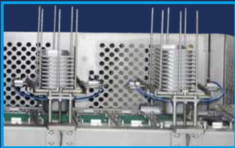
▲ Automatic 5-liter bulks destacking station
