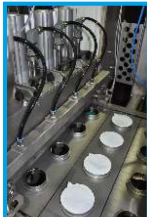
▲ Sealing stations for plastic film from the reel ▲
