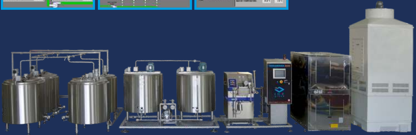
▲ Complete line with ageing tanks, dissolving unit, batch pasteurisation unit, homogeniser, control panel, ice water generator and water tower
