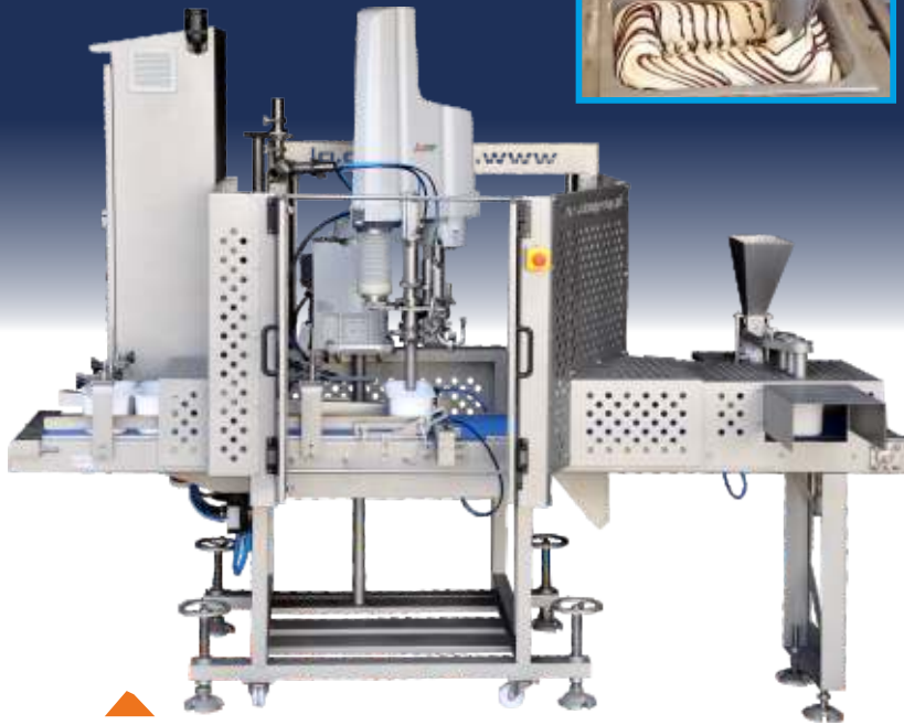
JUMBO ROBOT 4,5-axis version with belt conveyor
