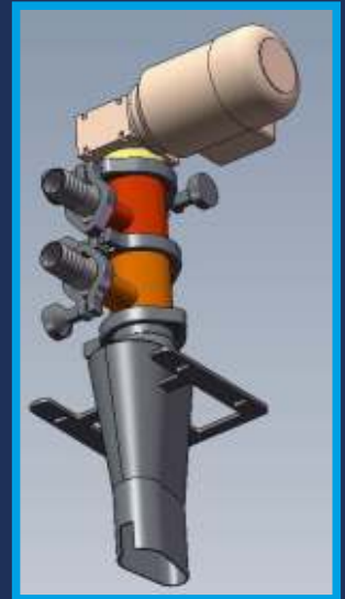
Cobra mixer for two ice cream colors or ice cream with syrup
