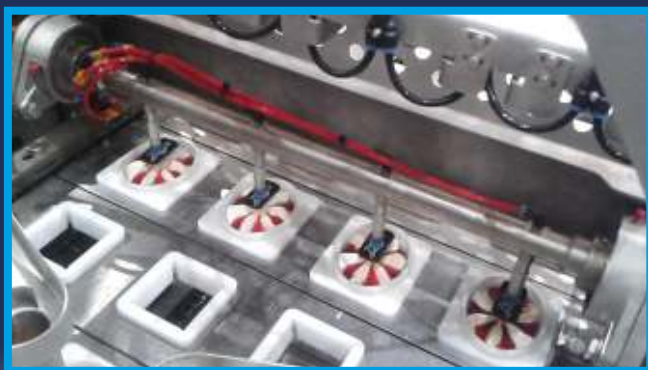
Automatic choco disk placing station
